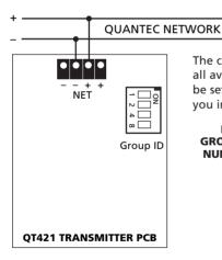
The chart below shows the DIP switch arrangements for all available RF Group IDs. The integrity transmitter must be set up with the same RF Group ID as the receiver(s) you intend to use it with.
